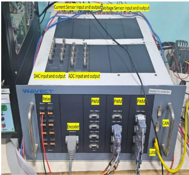
Fig. 9. Hardware setup of WAVECT controller.
