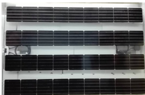
Fig. 3. Bifacial PV panel.
