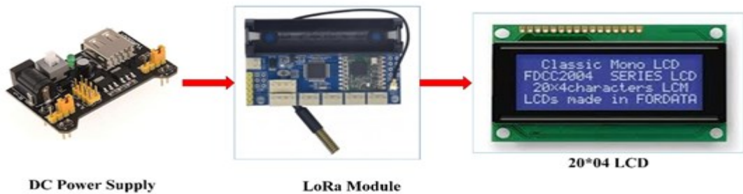
Fig. 4. Low cost PV monitoring system.
