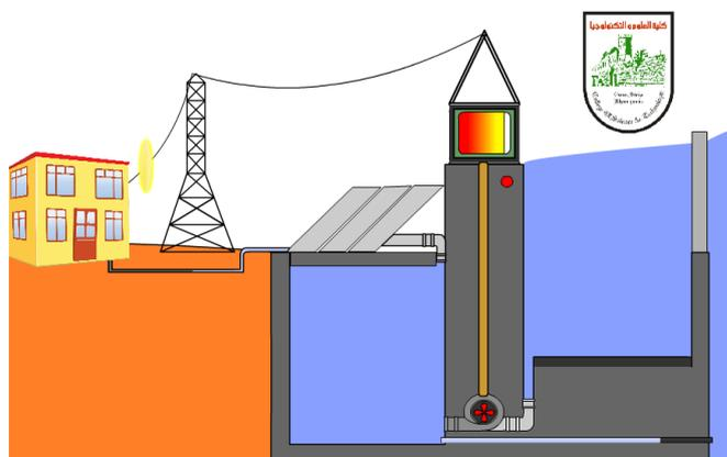
**Fig. 6.** A hyper station to produce power electricity from sea water and desalination.
