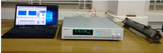
Fig. 5. Solar array simulator with resistive load
